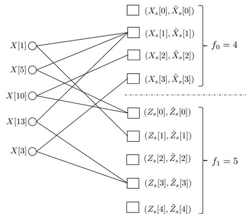
**Fig. 4:** A 2-left regular degree bi-partite graph, where the variable (left) nodes correspond to the unknown DFT coefficients and the check (right) nodes are the observations obtained through the FFAST architecture shown in Fig. 3, for the 20-point example signal  $\mathbf{x}$ . Each check node has two complex valued observations.
