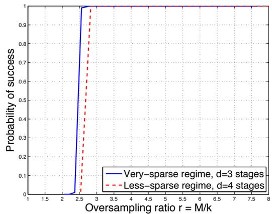
**Fig. 5:** The probability of success of the FFAST algorithm as a function of the oversampling ratio  $r$ . The plot is obtained for the two different sparsity regimes: i) the very-sparse regime and ii) the less-sparse regime. Each point in the plot is obtained by averaging over 10000 runs. Note that the oversampling ratio  $r < 4$  is sufficient for successful computation of the  $k$ -sparse  $n$ -point DFT using the FFAST algorithm.
